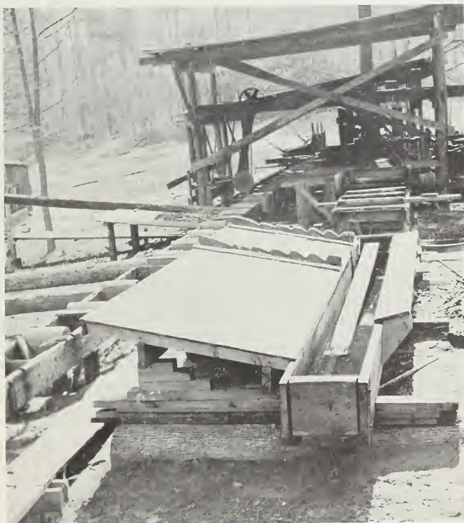
Figure 25. --Hand-dipping vat and drain board for applying antistain solution.
